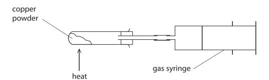
The copper powder in the test tube was heated strongly so that it could react with oxygen in the air in the apparatus.
