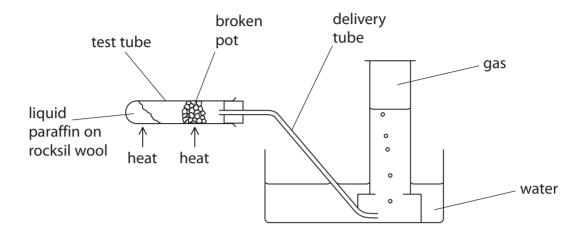
When the experiment is complete there is a danger that water will rise up the delivery tube into the hot test tube.
