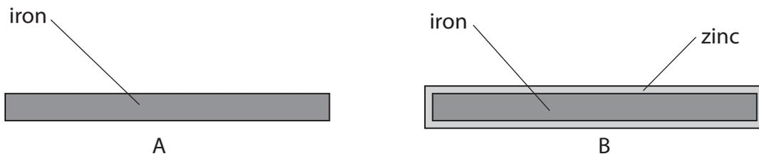
Sample B is coated with a thin layer of zinc.
