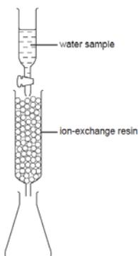
A 50 cm<sup>3</sup> sample of water containing dissolved calcium sulphate was passed through the ionexchange resin. Each calcium ion in the sample was exchanged for two hydrogen ions. The resulting acidic solution collected in the flask required 25 cm<sup>3</sup> of 1.0 × 10<sup>-2</sup> mol dm<sup>-3</sup> potassium hydroxide for complete neutralisation.
