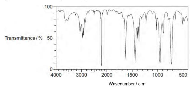
Identify **two** features of the infrared spectrum that support the fact that this is the infrared spectrum for but-2-enenitrile. You may find it helpful to refer to **Table 1** on the Data Sheet.
