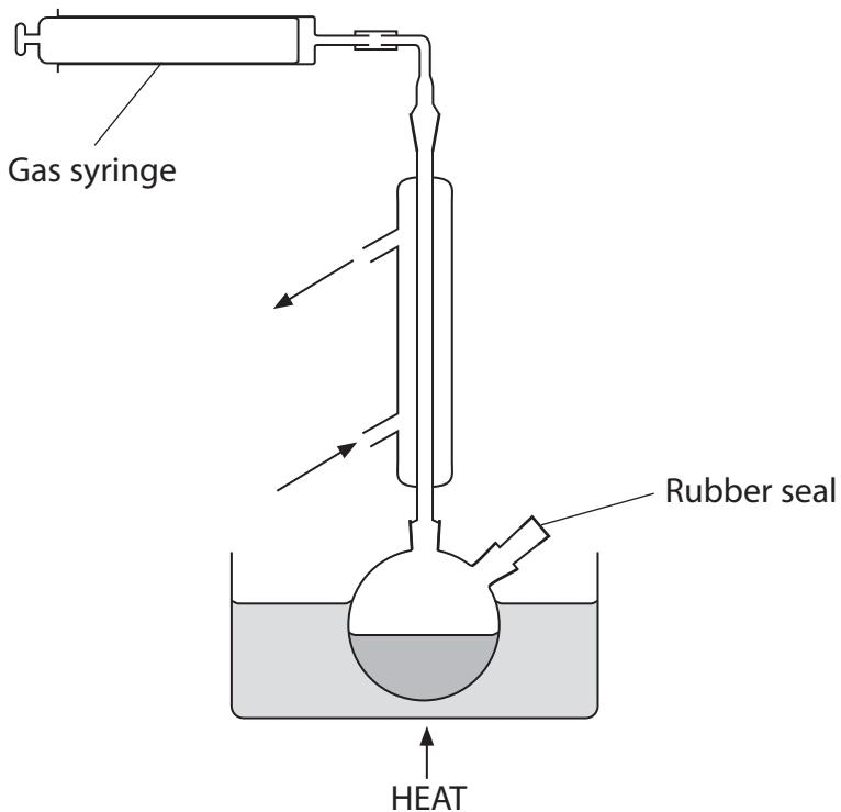
A solution of concentrated potassium hydroxide in ethanol was refluxed and the gas syringe connected as shown.
