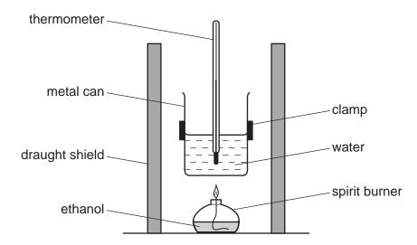
The ethanol in the spirit burner was burned to heat a measured mass of water in the metal can. The student recorded the initial and final mass of ethanol and the initial and final temperature of the water for each experiment.
