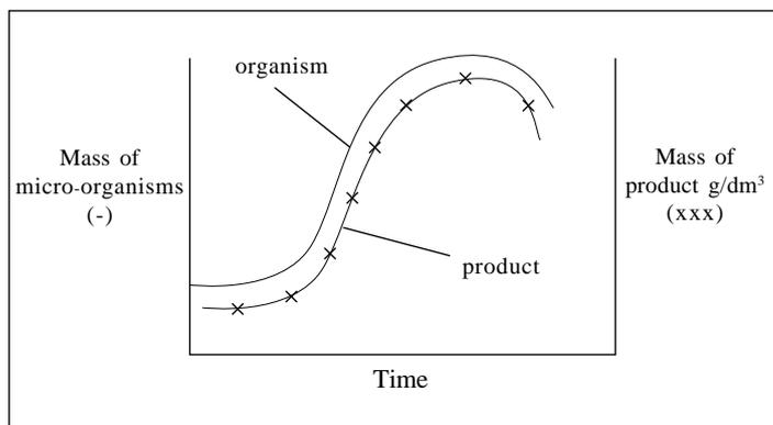
Fig 4 shows the typical growth and product curves for a micro-organism and its secondary metabolites.
