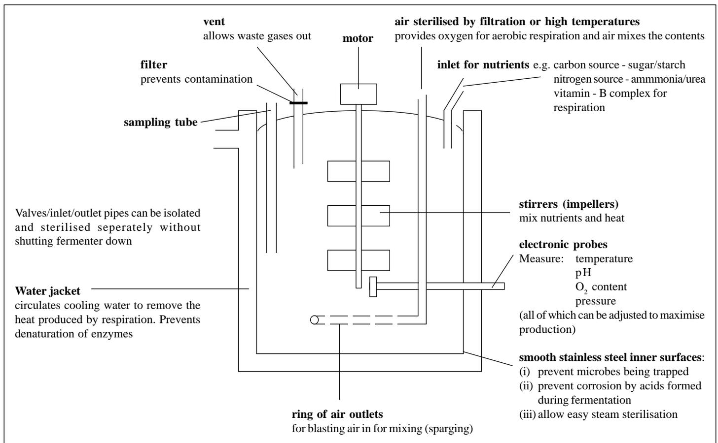
The aim of the process is to put the micro-organism - usually bacteria or fungi - into a sterile, carefully controlled environment (a steel tank) and supply it with the exact nutrients and conditions it needs to grow optimally. Usually, but not always this involves aerobic conditions. Under optimal conditions the growth of a micro-organism such as bacteria or yeast is shown in Fig 2.
