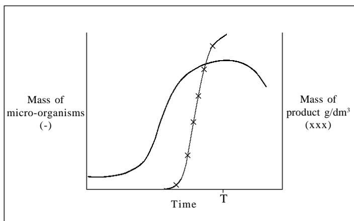
Note: Production of secondary metabolite starts when exponential growth stops and growth of cells starts to slow. Adding a lot of extra nutrients at time T (see graph) will simply increase the growth of the micro-organism but not formation of the product. However, by adding a small amount of extra nutrients at this time, the amount of product formed can be increased.
