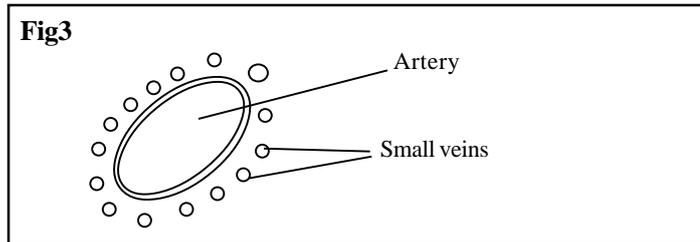
Tuna keep their most active swimming muscles 14°C warmer than the sea by using a countercurrent heat exchanger.
