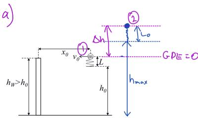
Conservation of energy:  $\frac{1}{2} k(\Omega L)^2 = mg \Omega h$   $\frac{\Delta h}{2} = \frac{1}{2} \frac{k}{mg} (\Delta L)^2$   $= \frac{1}{2} h mex = h_0 - \Delta L + \frac{k}{2} \frac{(\Delta L)^2}{mg} (\Delta L)^2$
