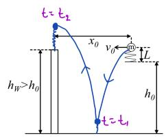
The above figure depicts a ball of mass m which is equipped on its lower side with a massless spring of uncompressed length  $L_0$  and spring constant k. The spring is initially compressed to a length  $L < L_0$ , as shown in the figure.
