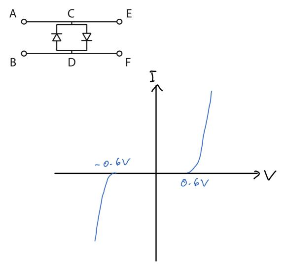
For small signals (low voltage), current doesn't flow through C-D. Amplifier operates.
