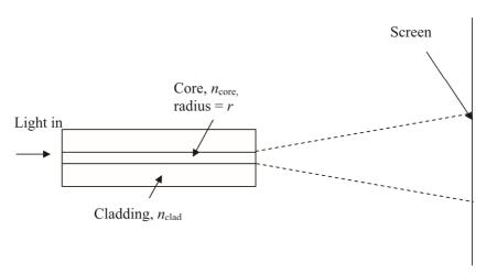
d) In an experiment, light is transmitted along the glass fibre before leaving at a perfectly vertical end. A screen is placed a long distance away from the end of the fibre and a uniform circular spot is seen as shown above. A small glass tank containing water is placed in front of the beam so it perfectly touches the end of the fibre. You may assume the tank is parallel to the screen. On a copy of the above diagram, sketch how the extent of the spot on the screen changes.
