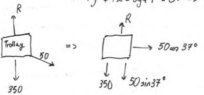
Newtons Second law upwards on trolley:  $R - 350 - 50 \sin 37^{\circ} = 0$  R - 350 - 50 (0.6) = 0 R = 350 + 30 = 380N
