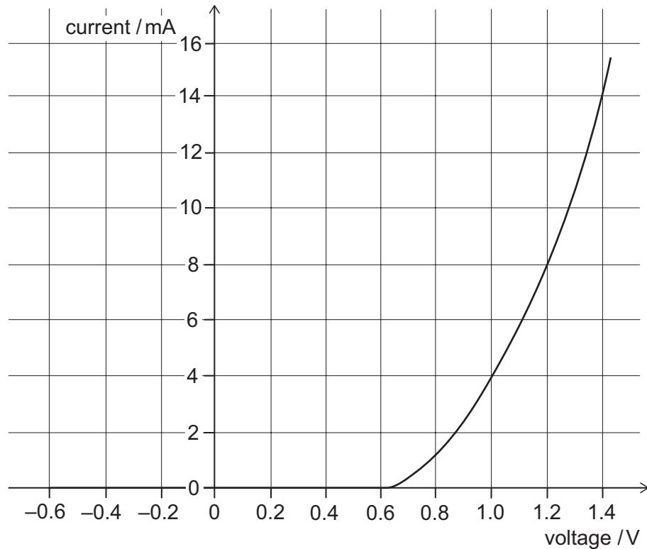
The diode is connected in series with a resistor and a 6.0 V battery. The current in the circuit is 8.0 mA.
