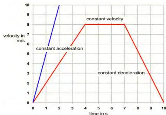
The following equations can be derived from velocity time graphs and are a useful alternative when solving problems which involve uniform acceleration:
