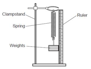
Li records the length of the spring for different weights on the spring, and plots the graph, as shown.
