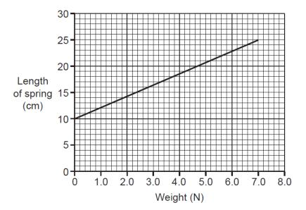
(i) The relationship for the spring can be expressed in the form L = mW + c, where L is the length and W is the weight.
