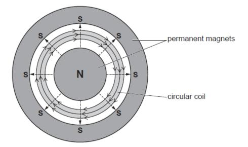
The direction of the magnetic field between the poles is shown as
