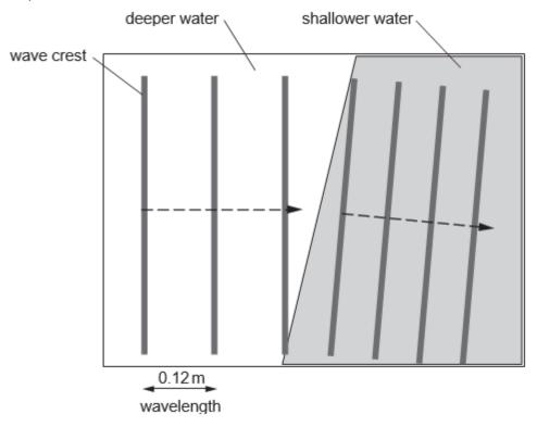
(i) The waves were produced at a frequency of 2.5 hertz (Hz).
