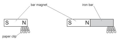
Describe the difference in magnetism between the bar magnet and the iron bar. [1] The bar magnet is a permanent magnet and the iron bar is an induced magnet
