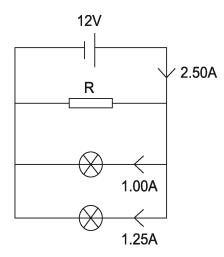
Calculate the power dissipated by resistor **R**.
