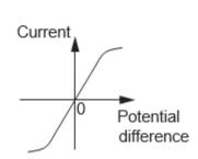
Which of the above shows the characteristic graph for a diode?
