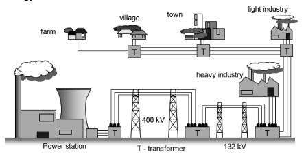
A step-up transformer is used in the National Grid.
