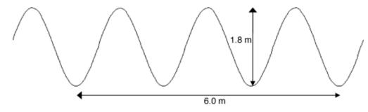
(i) The frequency of the wave is 2 Hz.
