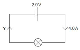
Write down the current flowing at point Y in the circuit.
