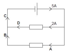
Which letter **A**, **B**, **C** or **D** shows the part of the circuit that carries a current of 2A?
