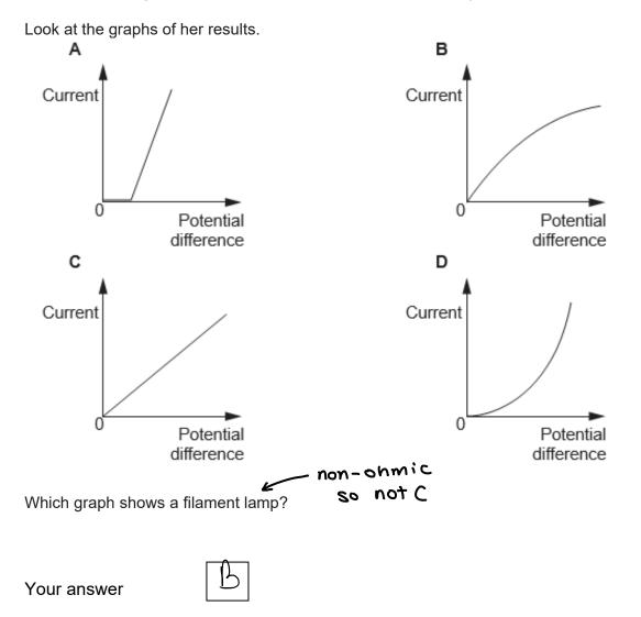
A student sets up four different circuits. He uses identical lamps and the same cell.
