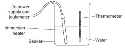
He heats up 1kg of water, using an immersion heater. He measures the temperature rise and calculates the specific heat capacity of the water.
