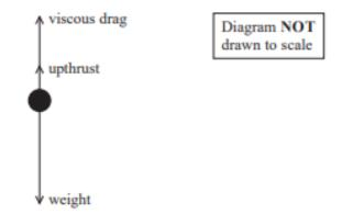
The raindrop is travelling at terminal velocity. The raindrop is spherical with a radius of 0.10 mm and a weight of  $4.1 \times 10^{-8}$  N.
