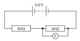
The reading on the voltmeter is 1.8 V.
