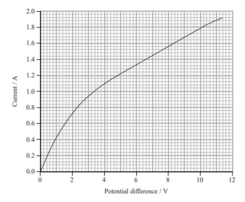
(a) Determine the resistance of the filament bulb when the potential difference is 7.0 V.
