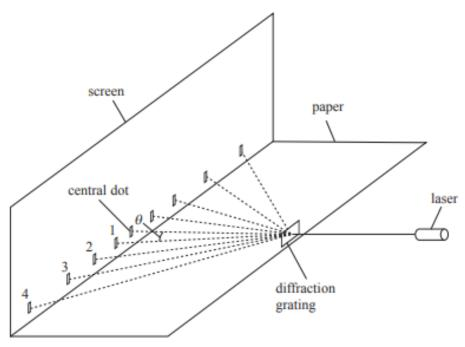
A laser light beam was shone at a diffraction grating. A series of dots of light was produced on a screen. The angles  $\theta$  between the light ray to the central dot and the light rays to the dots labelled 1 to 4 were measured with a protractor.
