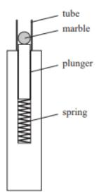
Determine the maximum possible launch velocity of the marble when the spring is compressed by 5.4 cm.
