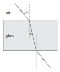
The student marks the path of the ray on paper. He takes corresponding measurements of the angle of incidence i and the angle of refraction r at the air-glass interface.
