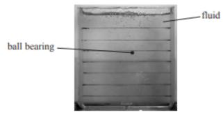
(a) To determine the viscosity  $\eta$ , the student used the equation  $v = \frac{d^2 g(\rho_b - \rho_f)}{18\eta}$
