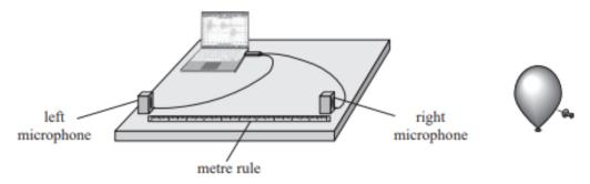
The computer was used to determine the time interval between the sound wave being received at the right microphone and being received at the left microphone.
