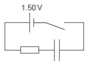
The cell has electromotive force (e.m.f.) 1.50 V and negligible internal resistance. The time constant of the circuit is 10s. The switch is closed at time t = 0. At time t, the potential difference across the resistor is 0.60 V.
