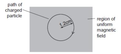
The direction of the magnetic field is perpendicular to the plane of the paper.
