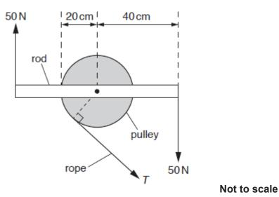
What is the moment of the tension *T* about the centre of the pulley?
