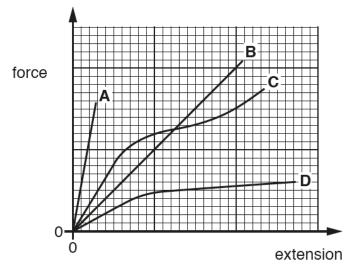
Which material is brittle and has the greatest ultimate tensile strength?
