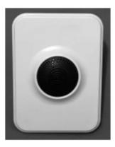
The mouse repeller produces ultrasound that repels mice but cannot be heard by humans. The mouse hears ultrasound directly and by reflection from the walls.
