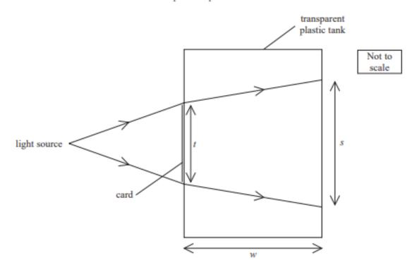
A rectangle of opaque card is stuck on the side of the tank containing the liquid. A light source is placed in front of the tank and the width s of the shadow of the card, which is formed on the back of the tank, is measured. The width t of the card and the width w of the tank are also measured.
