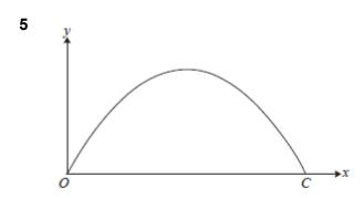
A particle P moves freely under gravity in the plane of a fixed horizontal axis Ox, which lies on horizontal ground, and a fixed vertical axis Oy. P is projected from O with a velocity whose components along Ox and Oy are U and V, respectively. P returns to the ground at a point C.
