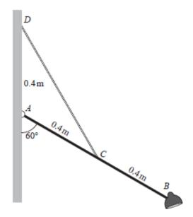
The diagram shows a wall-mounted light. It consists of a rod AB of mass 0.25 kg and length 0.8 m which is freely hinged to a vertical wall at A, and a lamp of mass 0.5 kg fixed at B. The system is held in equilibrium by a chain CD whose end C is attached to the midpoint of AB. The end D is fixed to the wall a distance 0.4 m vertically above A. The rod AB makes an angle of 60° with the downward vertical.
