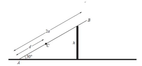
The diagram shows a ladder AB, of length 2a and mass m, resting in equilibrium on a vertical wall of height h. The ladder is inclined at an angle of 30° to the horizontal. The end A is in contact with horizontal ground. An object of mass 2m is placed on the ladder at a point C where AC = d.
