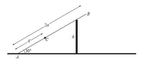
The diagram shows a ladder AB, of length 2a and mass m, resting in equilibrium on a vertical wall of height h. The ladder is inclined at an angle of 30° to the horizontal. The end A is in contact with horizontal ground. An object of mass 2m is placed on the ladder at a point C where AC = d.
