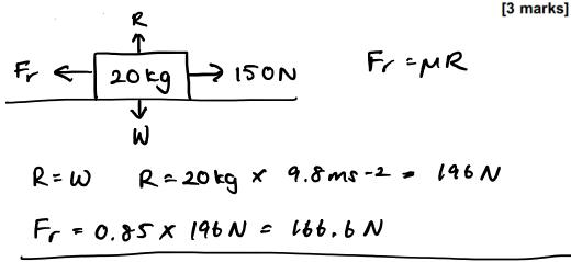
thrust force  $\angle$  friction force so crate (150N) remains stationary
