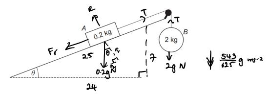
18 (a) B is released from rest so that it begins to move vertically downwards with an acceleration of  $\frac{543}{625} g\,\mathrm{m}\,\mathrm{s}^{-2}$
