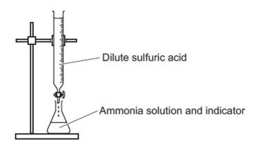
She adds an indicator to ammonia solution in a conical flask. She then adds dilute sulfuric acid from a burette until the indicator changes colour.
