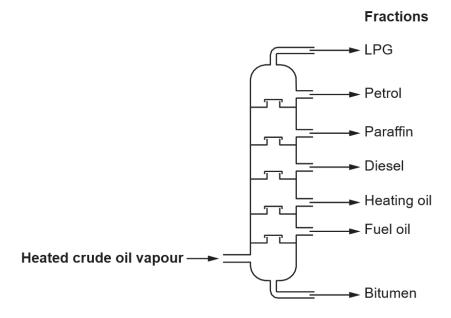
There is a temperature gradient in the tractionating column, with it being nottest at the bottom. Smaller hydrocarbons have a lower boiling point as there are weather forces between molecules. So, they condense higher up the column, separating from the vapour.
