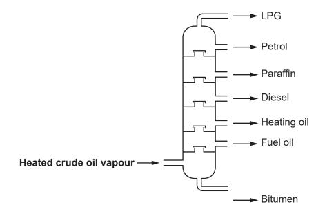
Explain why crude oil vapour can be separated by fractional distillation.
