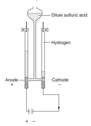
Hydrogen gas is made at the cathode.
