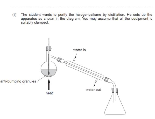
I. Anti-bumping granules were placed in the flask.
