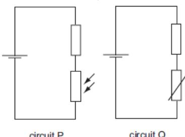
How does the potential difference across the fixed resistor in each circuit change when both the brightness of the light on the light-dependent resistor and the temperature of the thermistor are increased?
