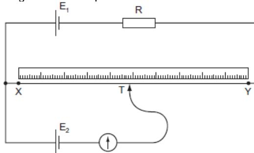
The contact T is placed on the wire and moved along the wire until the galvanometer reading is zero. The length XT is then noted. In order to calculate the potential difference per unit length on the wire XY, which value must also be known?
