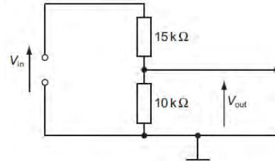
$V_{out}$  is equal to 4.8 V. What is the input voltage  $V_{in}$ ?
