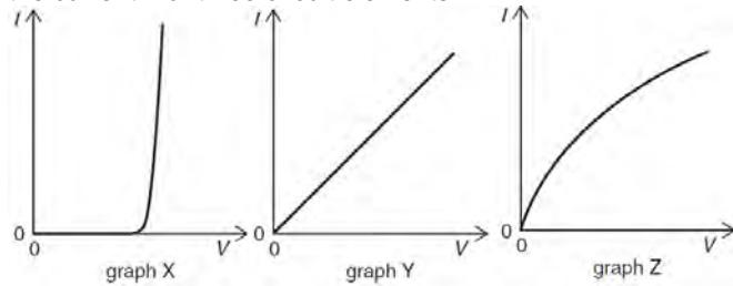
The three circuit elements are a metal wire at constant temperature, a semiconductor diode and a filament lamp.
