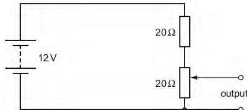
The fixed resistor and the potentiometer each have resistance 20 Ω. The circuit is designed to provide a variable output voltage. What is the range of output voltages?
