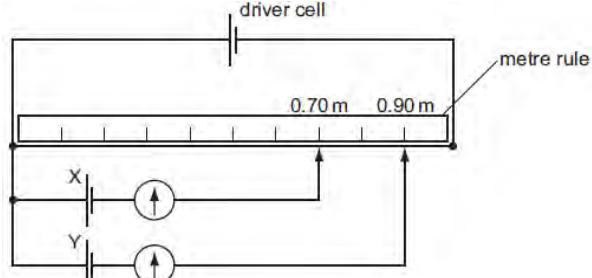
The balance points for cells X and Y are 0.70 m and 0.90 m respectively.
