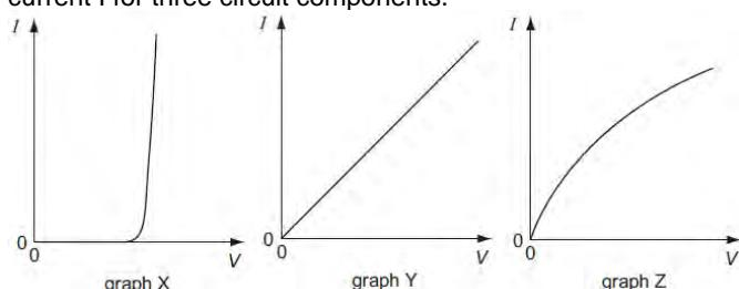
The components are a metal wire at constant temperature, a semiconductor diode and a filament lamp.
