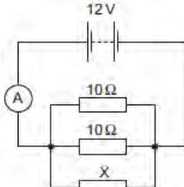
The battery has e.m.f. 12 V and negligible internal resistance. The ammeter reading is 3.2 A. What is the resistance of X?
