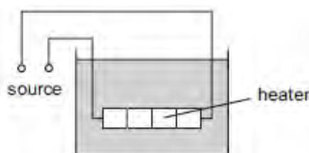
The heater has a resistance of 3.0  $\Omega$ . The voltage source has an e.m.f. of 12 V and an internal resistance of 1.0  $\Omega$ .
