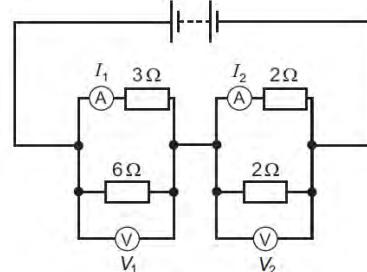
The readings on the meters are  $I_1$ ,  $I_2$ ,  $V_1$  and  $V_2$ , as labelled on the diagram.
