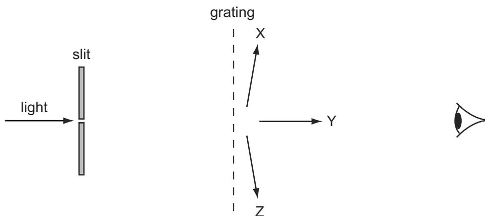
An observer views the slit through the grating at different angles, moving his head from X parallel to the grating, through Y, opposite the slit, to Z parallel to the grating on the opposite side.
