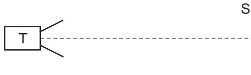
A small microwave receiver is moved from T towards S and receives signals of alternate maxima and minima of intensity.
