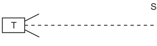
A small microwave receiver is moved steadily from T towards S and receives signals of alternate maxima and minima of intensity.
