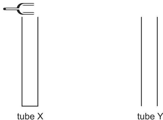
The tubes are identical except tube X is closed at its lower end while tube Y is open at its lower end. Both tubes have open upper ends.
