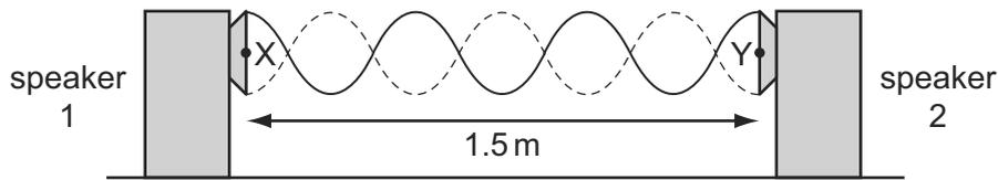
When a microphone is moved between X and Y, a distance of 1.5 m, six nodes and seven antinodes are detected.
