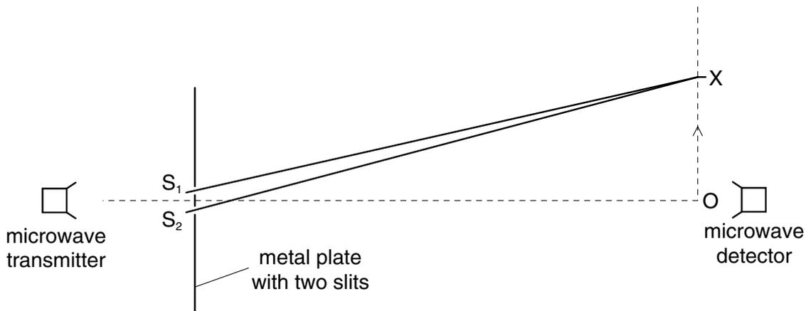
The detector is moved from O in the direction of the arrow. The signal detected decreases until the detector reaches the point X, and then starts to increase again as the detector moves beyond X.
