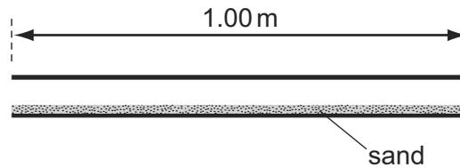
When a source of sound of a single frequency is put near one end of the pipe, the air in the pipe is found to resonate and a pattern in the sand shows that a standing wave containing three nodes is formed within the pipe.
