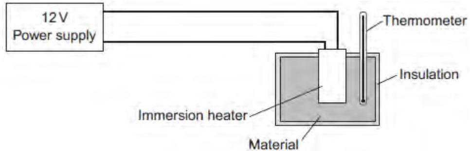
The student measured the time taken to increase the temperature of each material by 5 °C.
