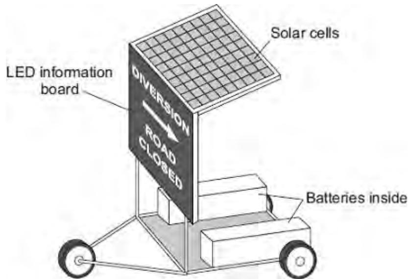
The batteries power the LEDs used in the information board.
