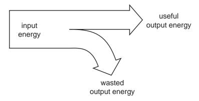
The device is 50% efficient.
