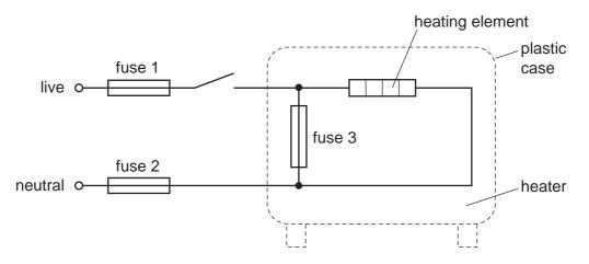
Which of the fuses are correctly placed?
