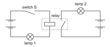
When switch S is closed, the relay operates. What is the state of the lamps?
