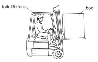
The force exerted by the fork-lift truck on the box is 3500 N upwards.
