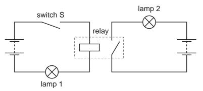
When switch S is closed, the relay operates. What is the state of the lamps?
