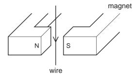
The current in the wire repeatedly changes between a constant value in one direction and a constant value in the opposite direction. This is shown on the graph.
