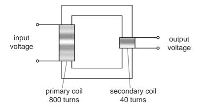
The input voltage is 240 V.
