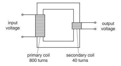
The input voltage is 240 V.
